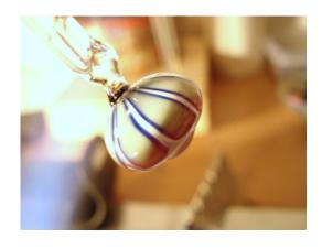
Melt off the thick clear rod and take away any excess glass with your tweezers.
