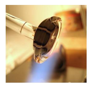
This is where heatcontrol comes in handy! Angel the cab a bit downward and point the flame on the bottom of the coil. Rotate slow! Once the clear starts to melt it will flow towards the center of the cap, dragging the dots along with it, getting the dots to meet in the center. Go slow! Add more clear if you need to, just remember only to add clear on the clear. Did I tell you to go slow?
