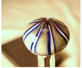
While the cab is still hot you might want to tap the bottom of your clear rod (yes, the one with the cab on!) on your work surface, making sure you hold the rod vertically. This flattens the cab a bit. Punty up the front of your cap with a clean (not scummy) thin clear rod.
